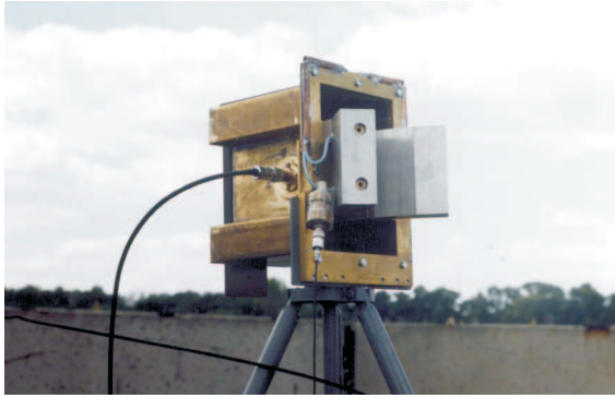
Fig. 11. Photograph of a plasma antenna H-waveguide exciter with HE cartridges installation platforms.
