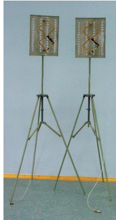
Fig. 13. The broadband antennas for recording RF emission of the plasma antenna.
