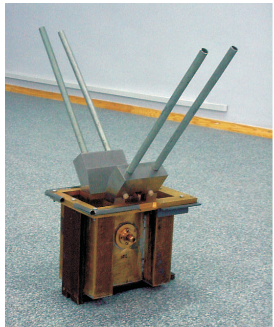
Fig. 9. General view of the four-jet plasma antenna prototype with the H-waveguide exciter.
