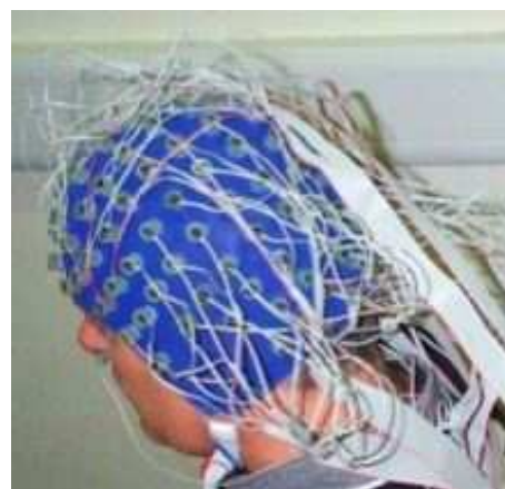
Fig. 2. The 10–20 configuration is the most common to obtain EEG data for diagnosis. The number of electrodes depends on the equipment available and the required precision.
